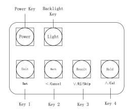
Keys are divided into three types including the short keys, long keys and key combinations. Long keys or key combinations (keys should be pressed and hold for 2 seconds) are used to realize the functions of Set, Cancel, RJ or Cal, and short keys are used to realize other functions.
