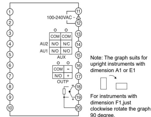
**Wiring graph for dimension D (72X72mm)instruments:**
