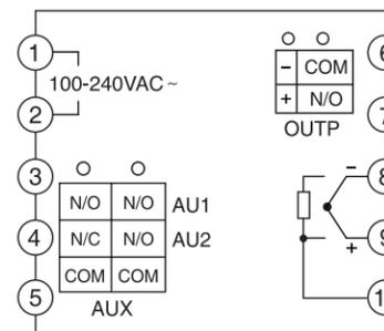
Note 1: Thermocouple should be directly connected to the back of the instrument wiring screws by compensation wires. No conventional conducting wires should be used in the input circuit. Pay attention to the correct type of compensation wires and polarity.
