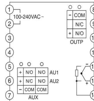
**Wiring graph for dimension D21 (48X48mm)instruments:**
